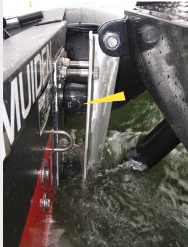
Seawater-resistant, robust TUBUS profile dampers made of co-polyester elastomer allow boats and crew to dock safely Wals Diving and Marine Service, 1970AC IJmuiden, Netherlands
