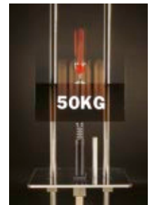
ACE demo showing a wine glass dropping free fall 1.3 m. Decelerated by a shock absorber not a drop of wine is spilled.
